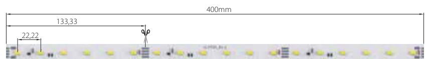
PT45R: 45pcs/m, 2 chips - FR4 PCB on - linear regulated 100mA - 24V - 18W/m - *2.025Lm/m
