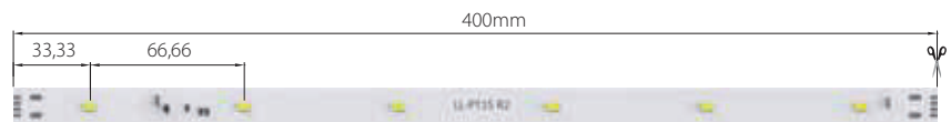
PT15: 15pcs/m, 2 chips - FR4 PCB on - linear regulated 100mA - 24V - 6W/m - *675Lm/m
